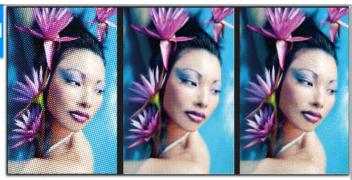
AM (traditional) most forgiving for production for higher quality need higher line screens FM (stochastic) - less forgiving, smaller dots appears like higher line screens
